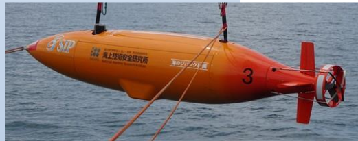
C-AUV#3, L=4m, W=545kg
